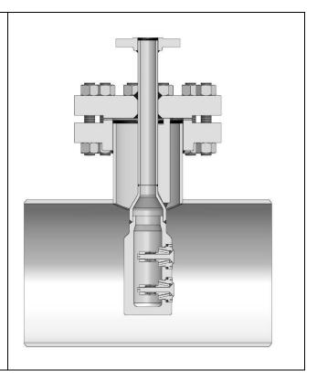
Spring Loaded Desuperheater: MODEL NO: SLD
